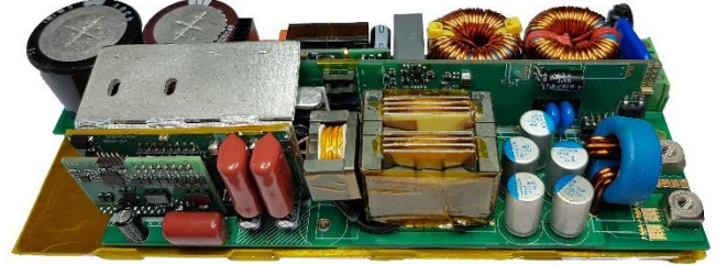
Fig. 18 1kW 12V AC-DC Power Supply 200mm x 80mm x 1U
