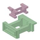
Figure 2 – showing "tunnel bobbin" design as may be used in resonant converters to achieve defined leakage inductance and provide for usage of unjacketed Litz wire.
