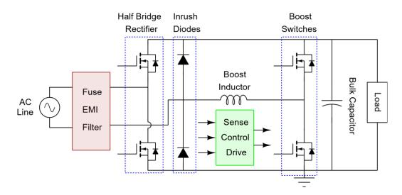
Figure 2 – "Totem Pole" Boost PFC Stage
