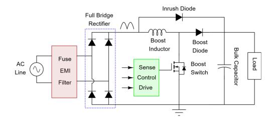
Figure 1 – Showing Boost Power Factor Correction Stage
