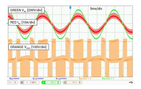
Figure 4 – Showing operational waveforms of the 3-level totem-pole PFC at 230Vac and 1.5kW. The switched node voltage in orange confirms that the inductor experiences significant lower volt-seconds as compared to that of a conventional (2 -level) PFC.
