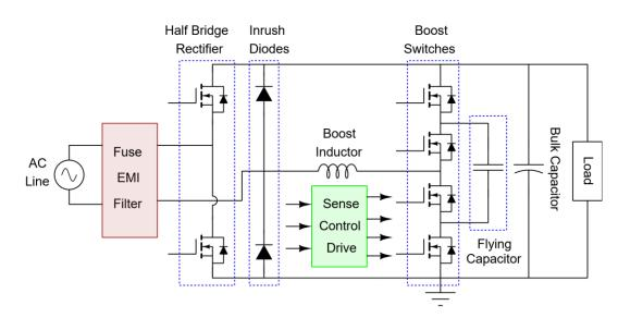
Figure 3 – Showing ICERGi multilevel "Stacked Multi-Phase" leg incorporated into totem-pole structure
