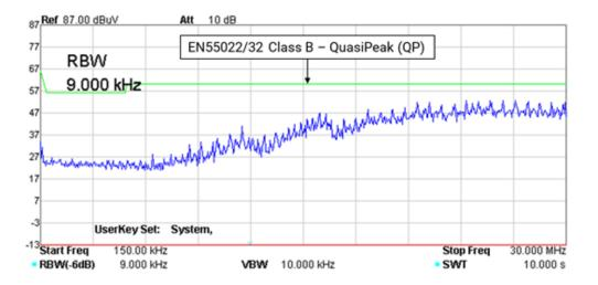
Figure 5 - Conducted EMI noise of the 3-level totem-pole PFC with two-stages EMI filters
