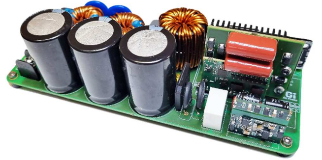
Fig. 8: 3kW bridgeless totem-pole PFC hardware prototype featured by ICERGi controller IC70101 and 8 x isolated gate drivers IC70101.
