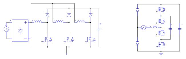
Fig. 1 Showing parallel nature of interleaved PFC (left) and stacked nature of Multilevel Approach
