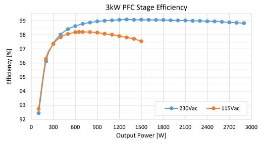
Fig. 4 "Extreme Efficiency" Full-Bridge Totem 3kW PFC-stage efficiency
