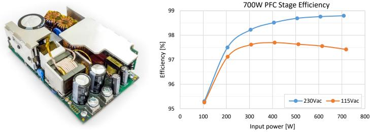
Fig. 3 700W full converter in 3"x5" footprint (left); 700W PFC stage efficiency (right);
