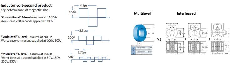
Fig. 2 Showing Magnetic Stress - volt-seconds (left) and size (right) reduction with Multilevel Approaches
