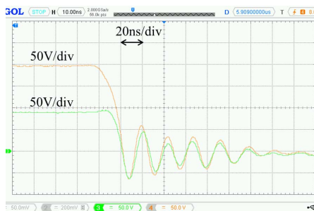
(c) Detailed turn-on transition
