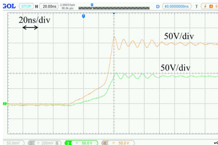
(b) Detailed turn-off transition
