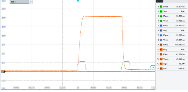
Fig. 4 Test conditions: R_{ON} = 3.3 \Omega , R_{OFF} = 2.2 \Omega , T_{pulse} = 105 \text{ ns} , V_{pri} = 9 \text{ V} ( V_{GS} , T_{pulse(on)} , T_{pulse(off)} )
